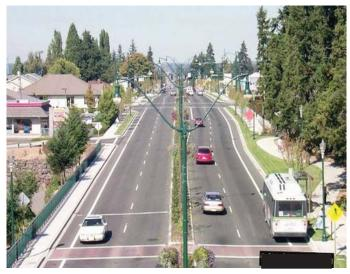
Figure 25 After (note: median, crosswalk, bus stop)
