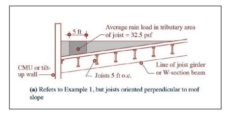
In a paper by Coffman and Williamson (2019) (see Ref. 7), they discuss that ponding can occur due to differences between "design slope" found in IBC, Chapter 15 and "roof slope" used in ASCE 7. Their concluding recommendation is: "When design constraints necessitate a 1/4 inch per 12 design slope be used, the framing members should be cambered or investigated for ponding."
