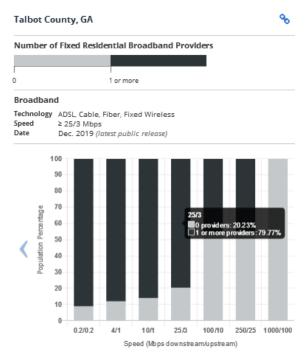
The chart shows the fraction of the population that has access to different numbers of residential broadband providers (the vertical axis) depending on the broadband speed (the horizontal axis) for the technologies selected to be displayed on the map. The majority of the county is rural and 78.65% of the rural area has at least one provider offering 25Mbs/3Mbs service. However, 21.35% of the rural population resides in areas that do not have even one provider.
