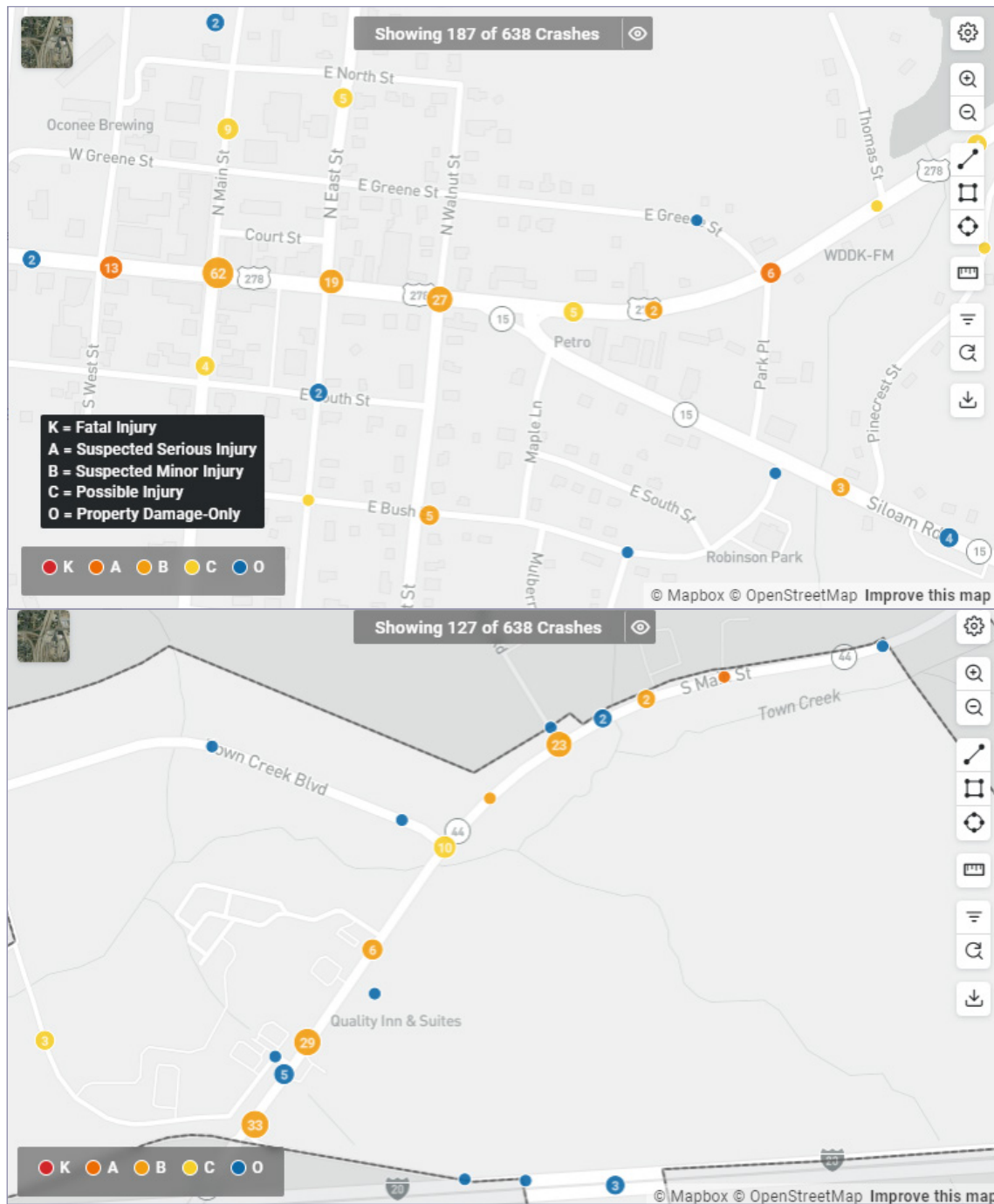
Figure 14. Approximate locations of vehicular crashes (2018–2022) in the two areas of Greensboro with the highest concentration of crashes: Downtown (top) and SR-44 north of I-20 (bottom). Each circle represents a cluster of crashes in proximity to the location indicated, and the color of each circle represents the severity of the most severe crash that occurred within that cluster (images from GDOT AASHTOWare).
