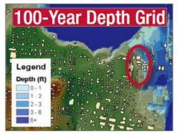
*Figure 1.* Example of Use of Depth Grids in Floodplain Mapping (not Floyd County)
