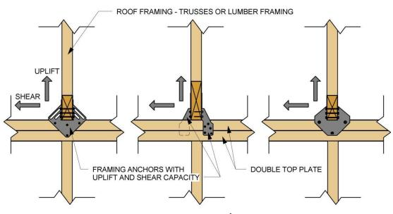
Figure AU402.2.4<sup>b</sup> Roof Framing to Wall Connection Detail
