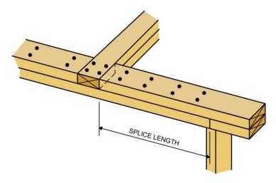
Figure AU402.2.10<sup>c</sup> Top Plate Intersection Detail
