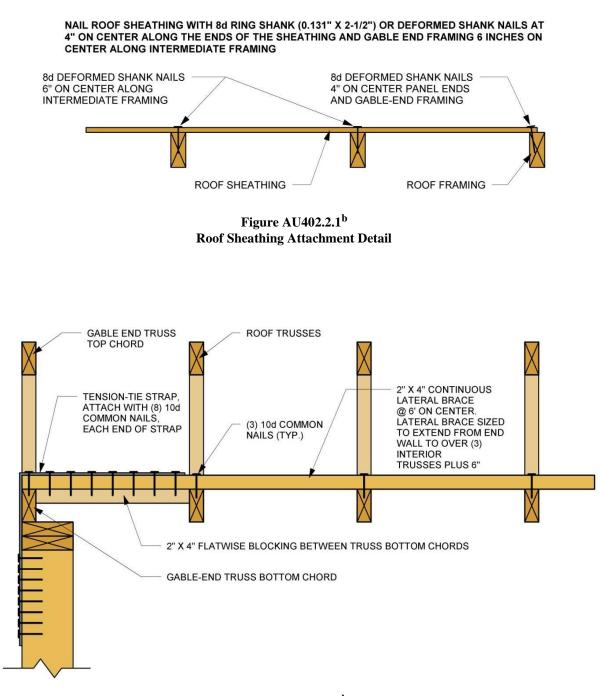
Figure AU402.2.2<sup>b</sup> Gable End Wall Connection Detail
