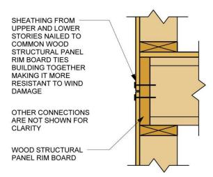
Figure AU402.2.5<sup>b</sup> **Sheathing Attachment at Elevated Floor Level Detail**
