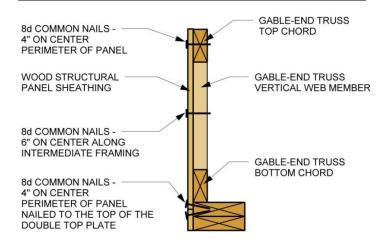
Figure AU402.2.3<sup>b</sup> Gable End Wall Sheathing Detail
