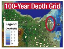
*Figure 1.* Example of Use of Depth Grids in Floodplain Mapping (not Burke County)
