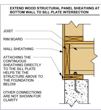
Figure 7-2: Wall Sheathing to Sill Plate Connection Detail (DRC Appendix R)
