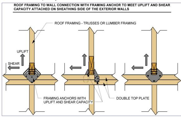
Figure 7-1: Roof Framing to Wall Connection Detail (DRC Appendix R)
