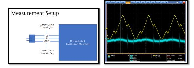
**Figure 2, Typical Microwave Oven Waveforms**
