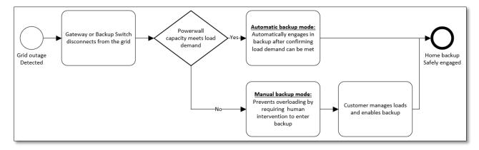
Figure 2: Example flow of Automatic and Manual Backup modes that ensure the system does not get overloaded upon transfer
