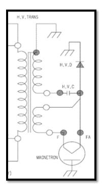
Figure 1, Typical Microwave Oven Circuit
