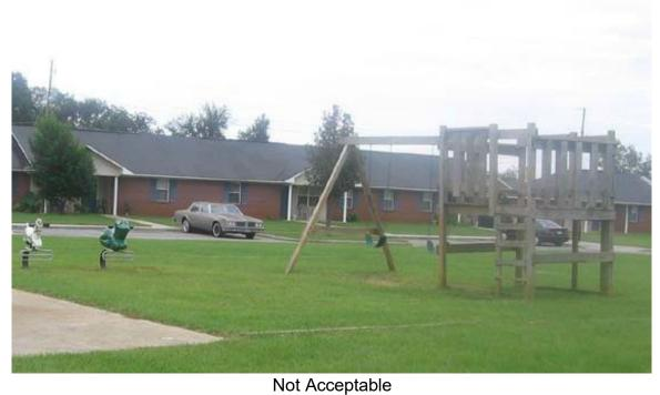
Equipment not constructed in compliance with CPSC guidelines for materials, ladder handrails, or ground cover. There is no observation bench.
