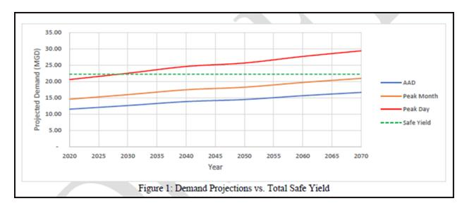
To ensure a reliable water supply the Water System is currently working to increase treatment capacity at the Crosstown Water Treatment Plant. This work will include production and infrastructure improvements to handle additional demand. The South Fayette Water Treatment Plant is designed for expansion to provide 18 MGD production. The Crosstown Plant may be high rated to 4 GPM/SQFT per filter upgrading the throughput of treatment to 18 MGD.
