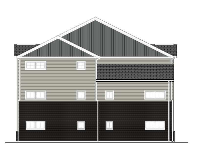
BUILDING #3 -SOUTH ELEVATION SCALE: 1/8" = 1'-0"
