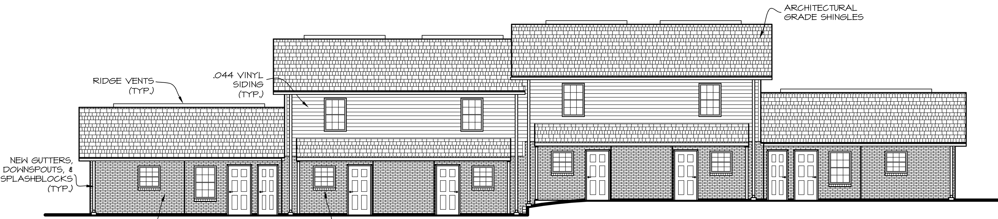
BUILDINGS "B & C" REAR ELEVATION
