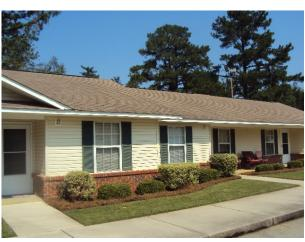
The buildings have a poured concrete foundation. The buildings have a combination brick and siding exterior, and a pitched roof covered with shingles.
