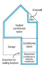
If supply registers deliver conditioned air to basement, it is considered conditioned. With no supply air, it is considered an indirectly-conditioned space.
