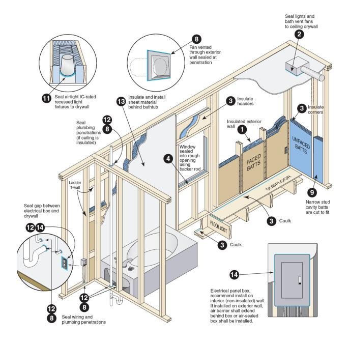
Disclaimer: This document is intended solely to This document is intended solely to help graphically demonstrate the air leakage provisions of section 402.4 of the 2009 IECC. It does not cover all airsealing locations or techniques. Other code provisions may be applicable as well.
