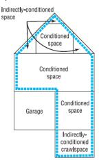
The top conditioned floor functions as a vaulted ceiling with interior walls althought it appears to have kneewalls and a flat ceiling. An advantage of this approach is that all upstairs ductwork is located inside the building envelope.
