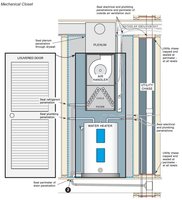
Disclaimer: This document is intended solely to rnis uocument is intended solely to help graphically demonstrate the air leakage provisions of section 402.4 of the 2009 IECC. It does not cover all airsealing locations or techniques. Other code provisions may be applicable as well.
