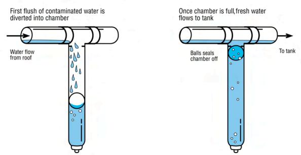
Figure 4.7 First Flush Diverter
