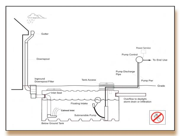
Figure 4.2 Diagram of below ground cistern
