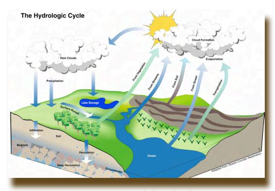
Figure 2.4 Basic Hydrological Cycle
