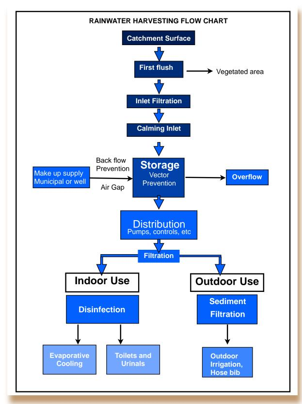
**Figure 4.3 Rainwater Harvesting Flow Chart**
