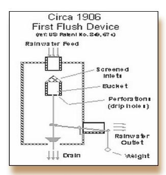
Figure 5.1 First flush diverter
