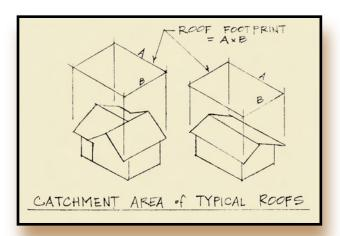
Figure 3.1 Catchment area of typical roofs
