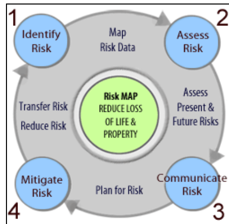
Figure 5. FEMA’s Risk MAP (Mapping, Assessment & Planning) lifecycle illustrates the process of identifying risks by utilizing flood hazard mapping and data
