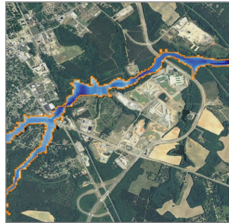
Figure 4. DCA can generate flood depth grids to illustrate the potential extent of flooding in a community
